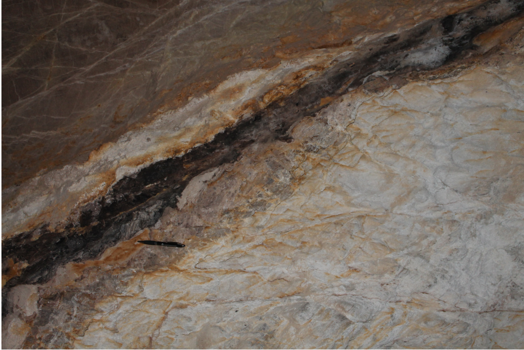
Fault with shale smear.
